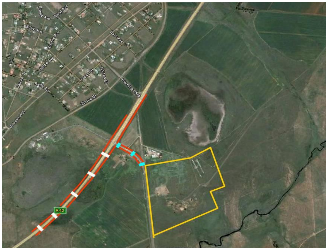
Layout of mitigation dykes and drift fence to protect migratory bullfrogs
